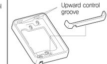
After attach the body supporter with 2screws, insert the upward support into the upward groove of body supporter, and then fix it with a screw.
