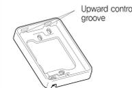
After attach the body supporter with 2screws, put the Door Camera into the grooves of body supporter, and then fix it with a screw.
