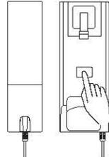
To release the door, press the "Door open" button during the communication.
