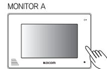
Press and hold [Door/Interphone] button for 2 seconds.
