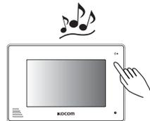
Monitor speaker rings the calling sound, and call is connected when pressing [Talk/Menu] button one more time. (Talking time : 3 minute).
