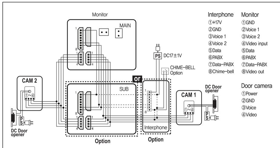
※In case of a single house application, an extra 17V(±1V) adaptor is necessary for the extended interphone.
