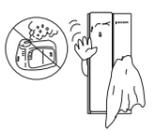
Keep away from humidifier and stove. High temperature and humidity can cause malfunction
