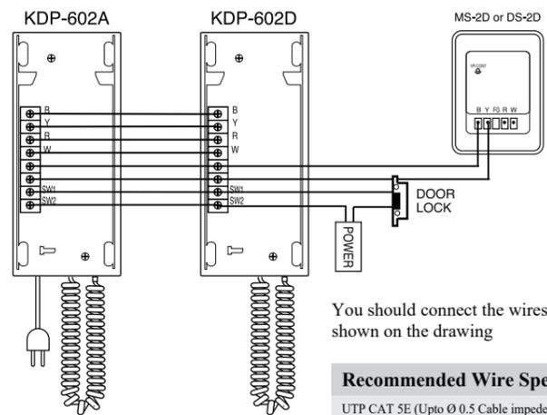
You should connect the wires as shown on the drawing
