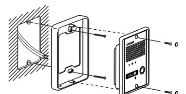
After attaching the body supporter with 2screws, put the Door Camera into the grooves of body supporter, and then fix it with screws.
