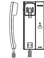
Pick up the handset and communicate with a visitor. After end of communication, return the handset where it is locked
