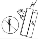
As this device consists of precise electronic components, and high voltage is generated internally, do not attempt to disassemble.
